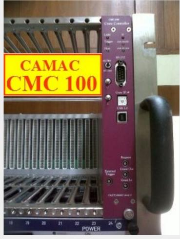
CAMAC system The controller is the right most module Addressing scheme is N,A,F 1  $\mu$  s/word
